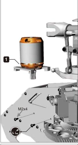
When installing the pinion confirm the position of pinion/ main gear as pictured below.
