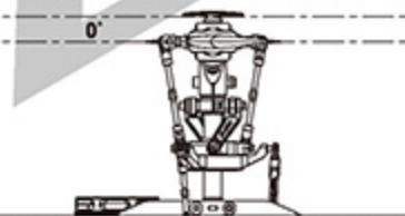
Stick Position at Middle/Throttle 90%/Pitch 0° 搖桿中速/油門90%/Pitch 0°
