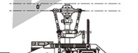
Stick Position at Middle/Throttle 90%/Pitch 0° 搖桿中油門90%/Pitch 0°
