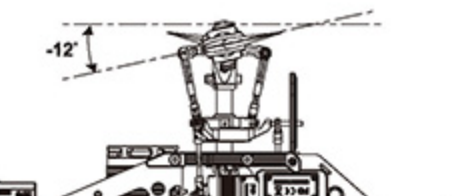
Stick Position at Low/Throttle 100%/Pitch -12° 搖桿低油門100%/Pitch-12°
