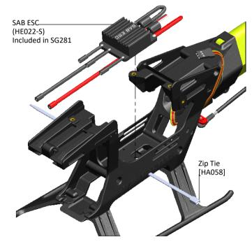
**Note:** Make sure to secure the ESC in place with a zip tie.
