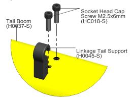
Socket Head Cap Screw M2.5x6mm
