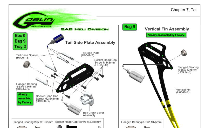
Socket Head Cap Screw M3x8mm
