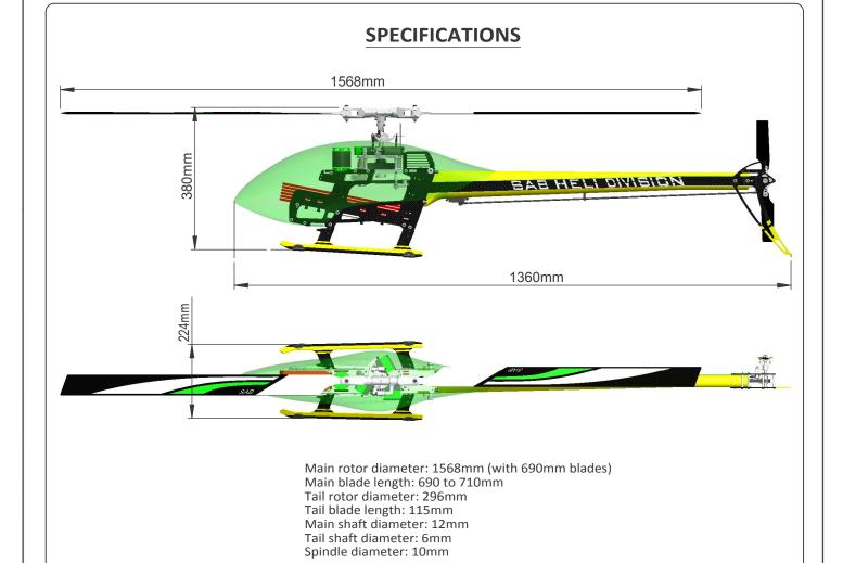
Weight including standard electronics: 3290g (excluding batteries). Motor size: Maximum 64mm diameter, maximum height 64mm Battery compartment: 60x58x350mm (adaptable to 64x58x350mm)
