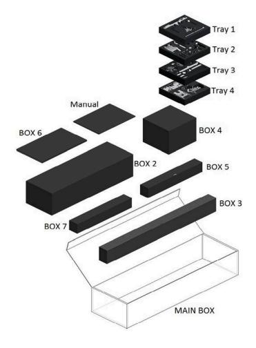
The assembly process is described in the following chapters of this manual. Each phase begins with a green frame which gives the box, the bag with screws (and miscellaneous items), and the foam tray with the components required for the phase.
