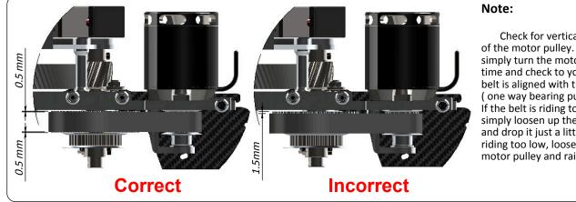
Check for vertical alignment of the motor pulley. To do this, simply turn the motor several time and check to you see if the belt is aligned with the big pulley (one way bearing pulley). If the belt is riding too high, simply loosen up the motor pulley and drop it just a little bit, if it is riding too low, loosen up the motor pulley and raise it a bit.
