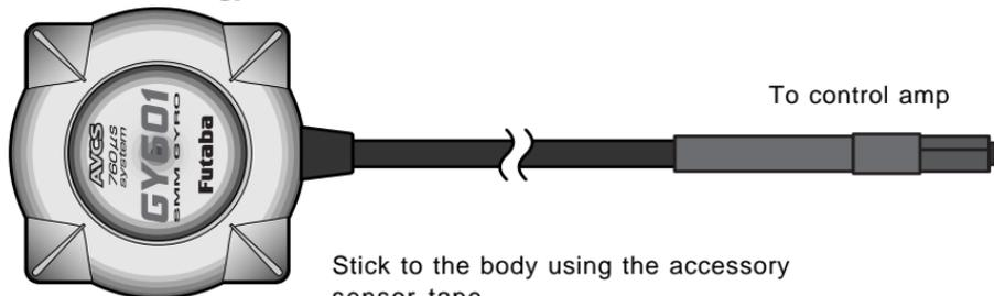
Stick to the body using the accessory sensor tape.
