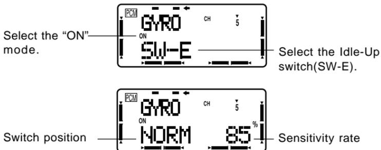
Set the "NORM", "IDL1" and "IDL2" gains at each setup screen.
