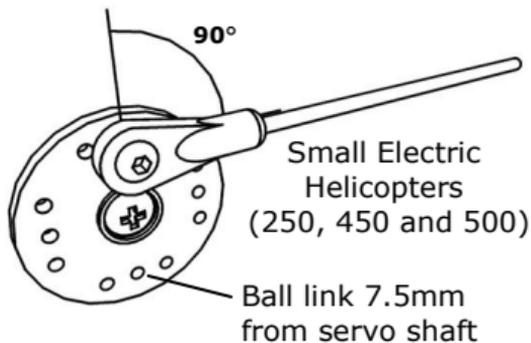
Follow the advice in the helicopter's assembly manual regarding the placement of the ball link onto the tail servo horn. When such advice is not provided or has resulted in poor tail performance we recommend placing
