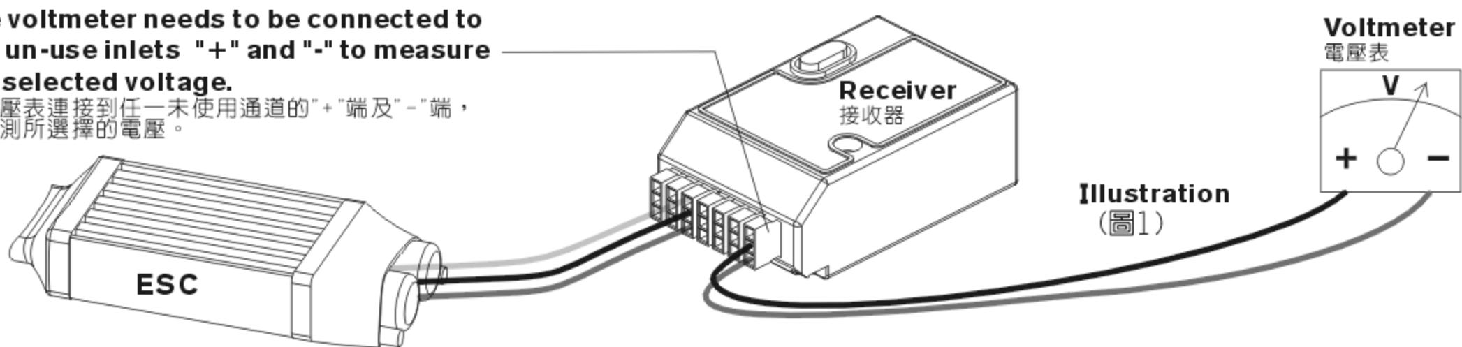
**NOTE:** Certain servos are designed to work with high voltage, while other servos are designed for lower voltage.
