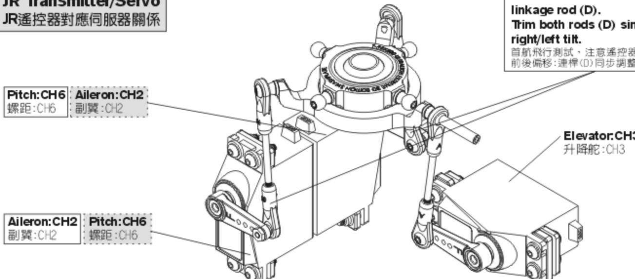
Please note to set the subtrim neutral for the first trial flight. If the helicopter wags, please trim linkage rod (D). Trim both rods (D) simultaneously to adjust for forward/backward tilt. Trim rod (D) separately for right/left tilt.
