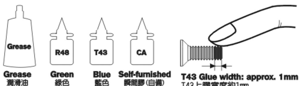
R48 metal tubular adhesive (eg. Bearings). T43 thread lock, apply a small amount on screws or metal parts and wipe surplus off.
