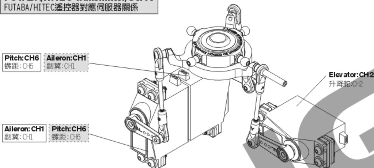
Positions of CH1、CH6 are exchangeable, After assembling as photo (Note: Set the transmitter under CCPM 120 degrees mode), pull throttle stick (pitch) upward. If one swashplate servo (or two servos) moves downward, adjust reverse switch (REV) on the transmitter to make it moves upward. If three servo move downward, adjust the travel value (+-) of SWASH CH6 on the transmitter to make them move upward. When the actions of Aileron and Elevator are opposite, adjust travel values of SWASH CH1 and CH2.
