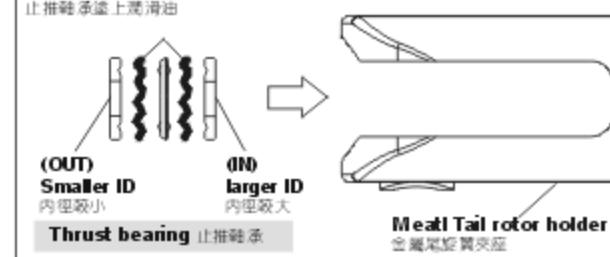
Thrust bearing 止推轴承
