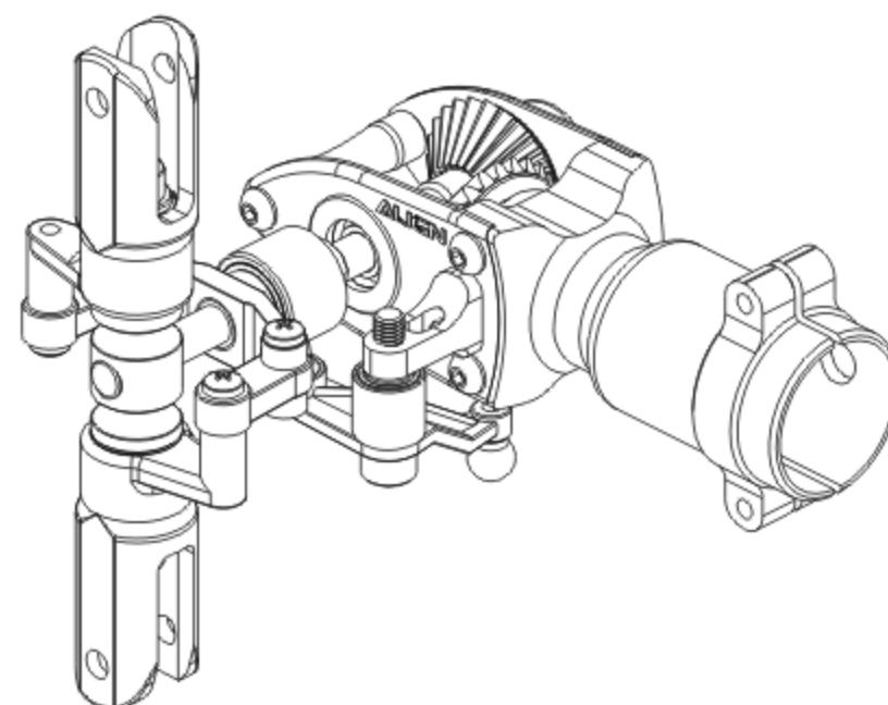
Apply a little amount of T43 thread lock when fixing a metal part.
